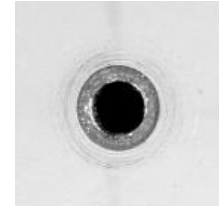
Shiny ring around the bore hole
