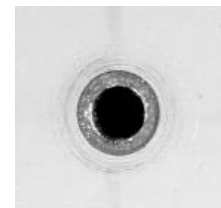
Shiny ring around the bore hole
