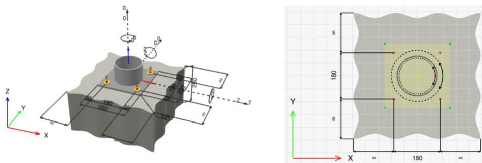
Fig. 6.53: Baseplate connection using post installed chemical anchors
