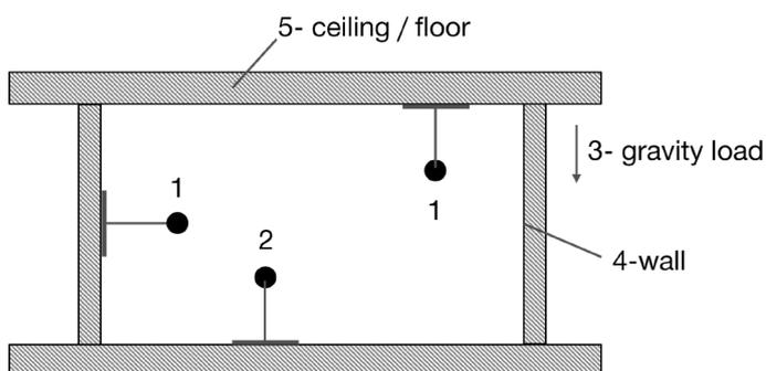
Fig. 6.35: Model showing vertical effect of seismic action
