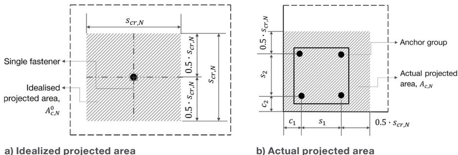
Fig. 6.17: Geometric influence area considered in cone break-out failure
