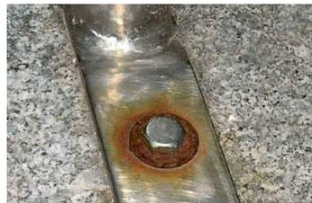
b) Heavy corrosion of a zinc plated carbon-steel washer
