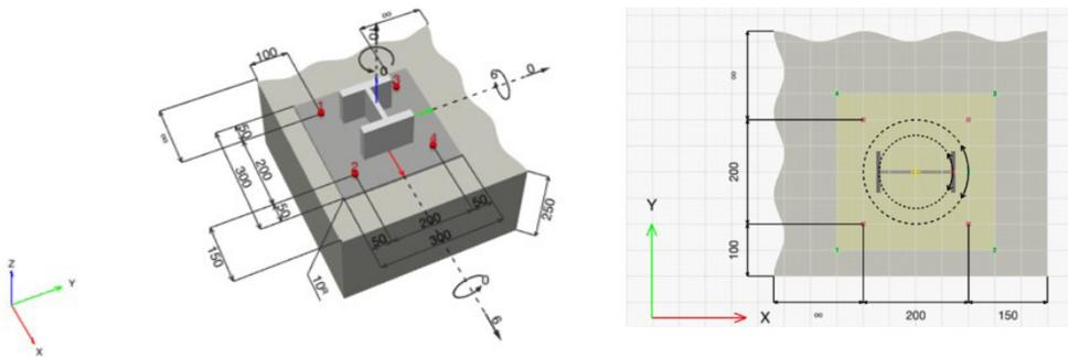
Fig. 6.24: Baseplate connection using post-installed mechanical anchors
