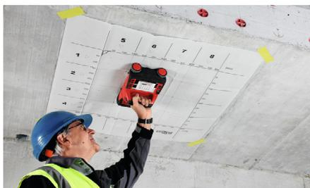
c) Scanning for ferrous and non-ferrous objects
