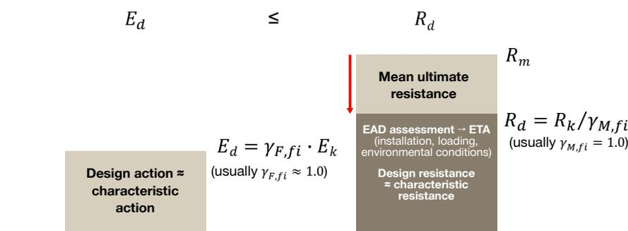
Fig. 6.39: Load vs resistance concept in fire design
