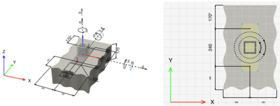
Fig. 6.37: Baseplate connection using post-installed chemical anchors
