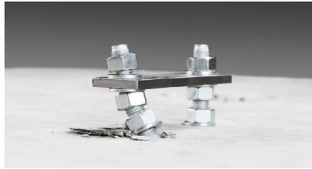
b) Failure with lever arm
