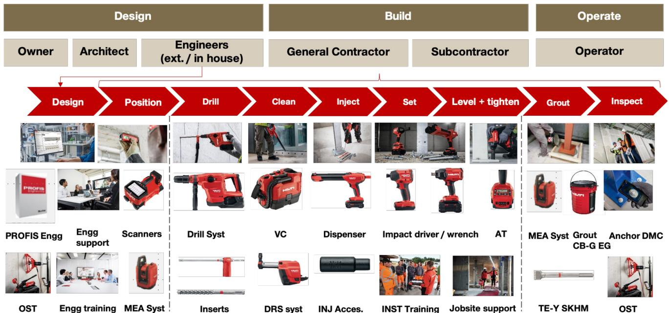
Fig. 8.2: Flowchart for installation of post-installed anchors
