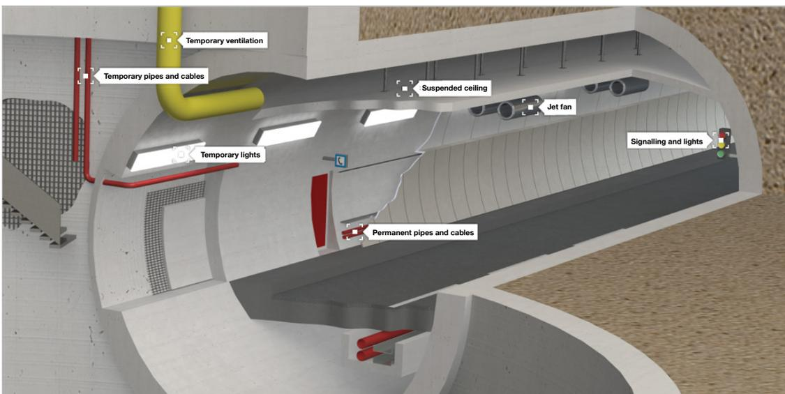
Fig. 2.4: Illustration of typical applications for tunnel structures
