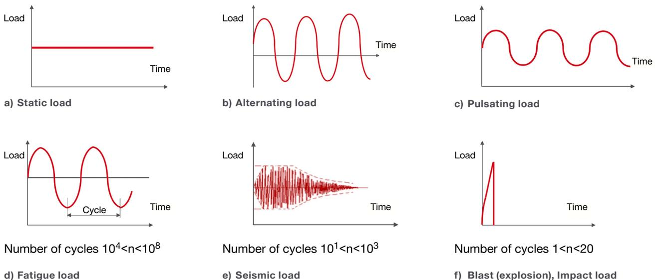
Fig. 3.12: Different loads / actions experienced by anchors
