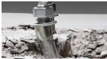
Fig. 3.22: Concrete pry-out failure under shear loading
