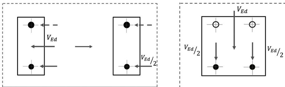
← - - Load distribution to the anchor is not considered for concrete edge failure verification
