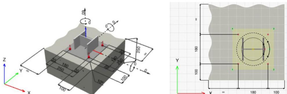
Fig. 6.29: Baseplate connection using post-installed mechanical anchors
