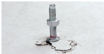
Fig. 3.17: Pull-out failure in tension
