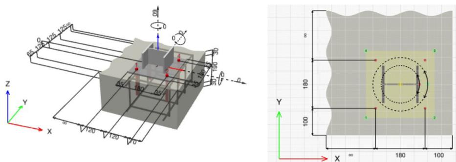
Fig. 6.31: Additional supplementary reinforcement in concrete base material
