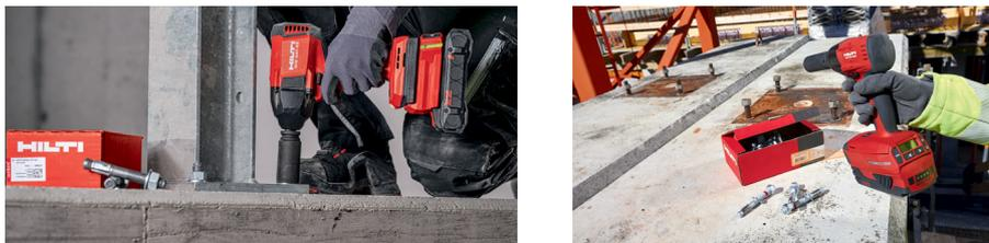
Fig. 8.16: SIW system torque wrench and AT module
