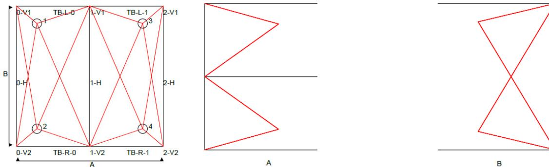
Fig. 6.32: Strut-and-tie model
