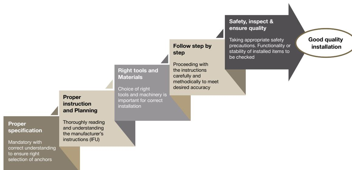
Fig. 8.1: Key points to be followed for proper installation
