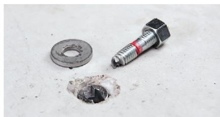
Fig. 3.15: Steel failure under tension loading
