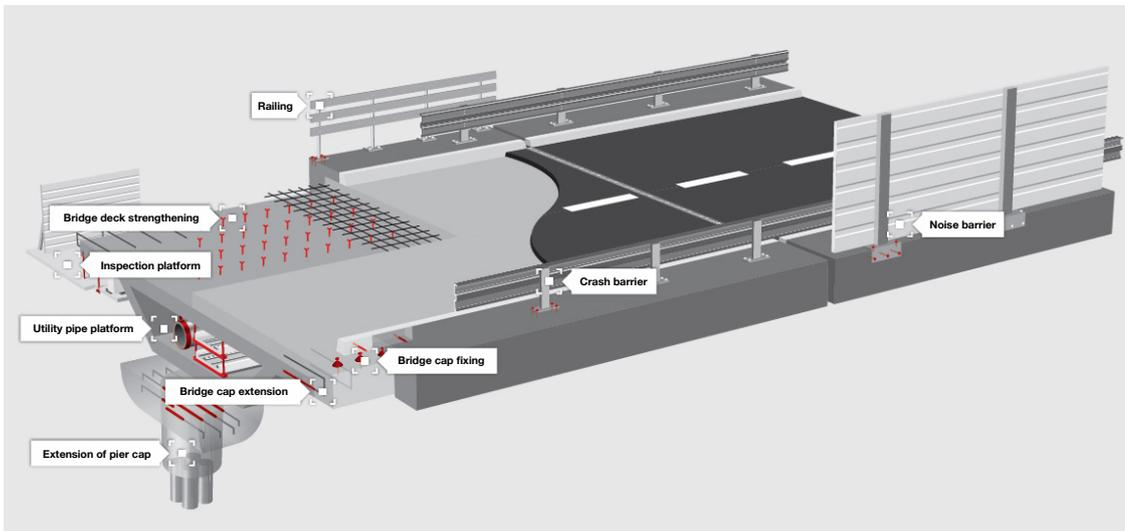
Fig. 2.3: Illustrations of typical applications for jobsite bridges
