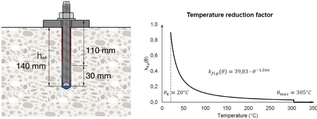
Fig. 6.50: Temperature profile considered in Simplified method
