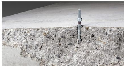
Fig. 3.23: Concrete edge failure under shear loading
