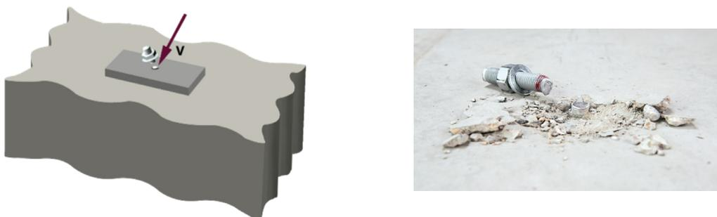
a) Failure without lever arm
