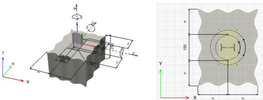
Fig. 6.46: Baseplate connection using post-installed mechanical anchors
