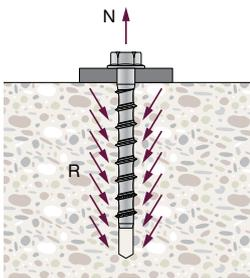
Fig. 3.7: Screw anchor
