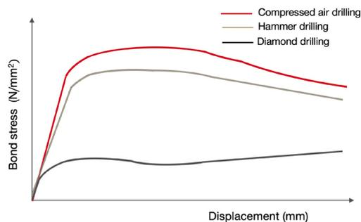
Fig. 3.25: Bond stress-displacement graph for bonded anchors in cleaned holes with hammer and diamond drilling ([2]), example of a system not suitable for diamond coring.
