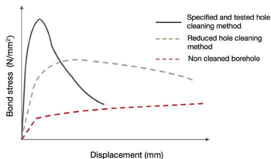
Fig. 3.26: Load displacement curve for well-cleaned / uncleaned holes in cracked concrete ([2])
