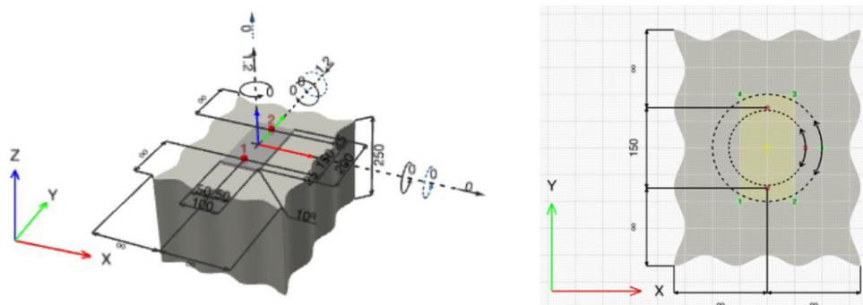
Fig. 6.48: Baseplate connections using post-installed chemical anchors
