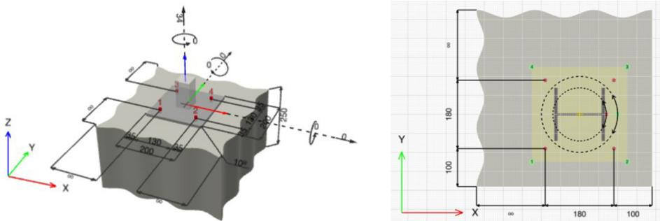
Fig. 6.26: Baseplate connection using post-installed concrete screw anchors
