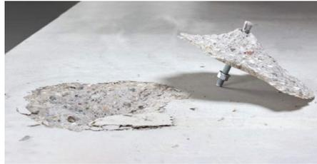
Fig. 3.16: Concrete cone failure under tension loading
