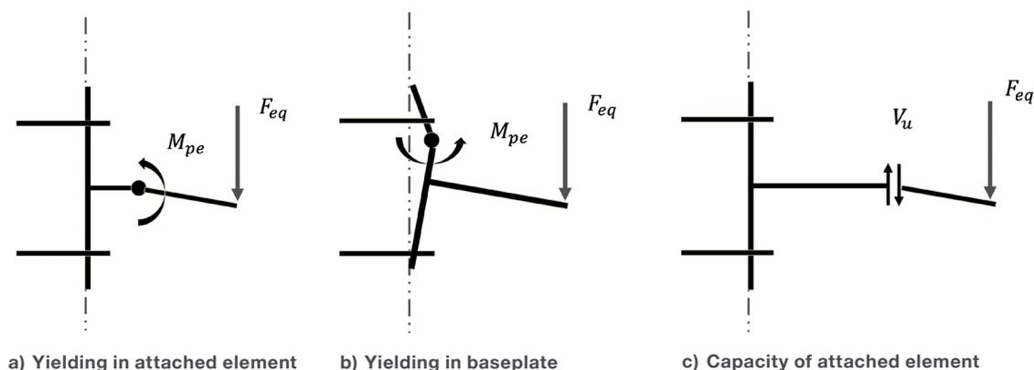
Fig. 6.36: Seismic design by protection of fastening
