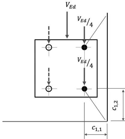
Fig. 6.10: Shear load acting parallel to the edge
