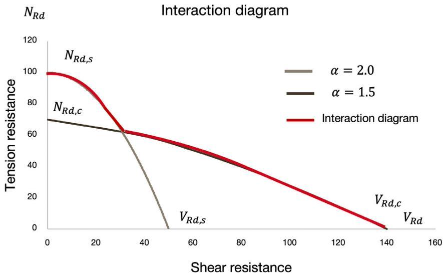
Fig. 6.23: Interaction between tension and shear diagram
