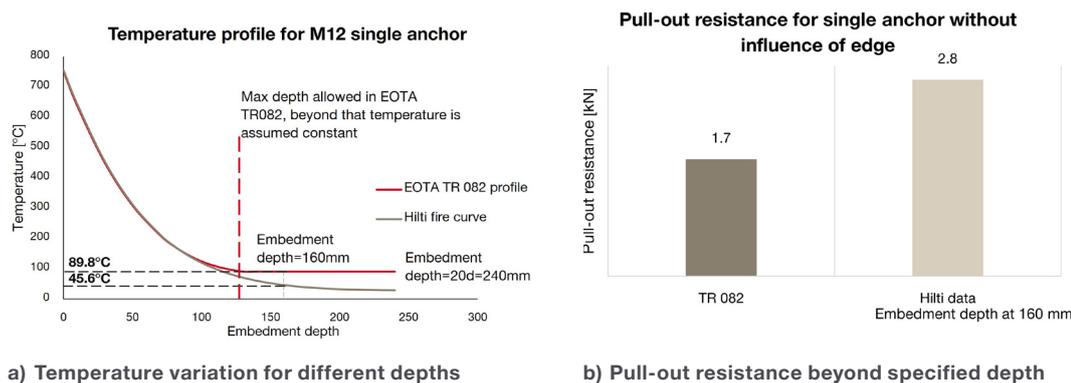
**Note:** Pull-out resistance has been calculated for HIT-RE 500 V4 anchor as per ETA 20/0541.
