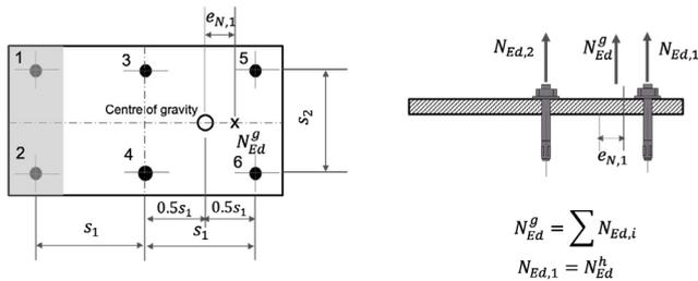
anchors 1 and 2 are in compression and hence neglected. anchors 3 to 6 are considered as group under tension loading. anchors 5 and 6 experience the highest loads due to the eccentricity.
