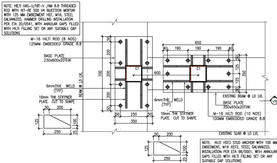
Fig. 8.20: Reference specification for post-installed anchor solution
