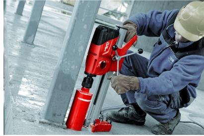
b) Diamond core drilling machines
