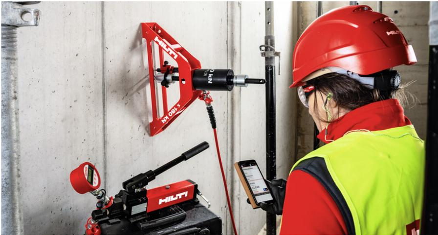
Fig. 8.19: Onsite testing by Hilti (unconfined tension setup)
