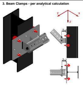
Transition of the forces generated on inclined brace to base material connector's coordinate system
