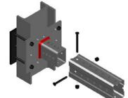
3. Base plate and through bolts - per analytical calculation
