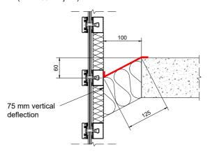
Maximum Movement Capability: ± 25 % horizontal and vertical movement, see above table for min, joint width recommendations to suit specific movement requirements. Please note, these are different and not to be combined. For combined movement, please contact Hilti for further support.
